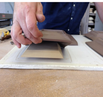
12. Release from Form with one finger when stiff leather hard.
