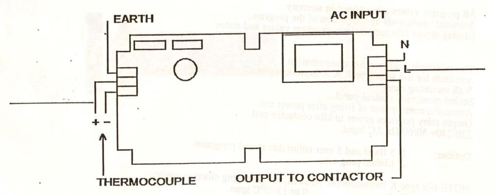
Note. The contactor output is a switched AC Live supply.
