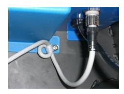
ATTACH A ZIP TIE TO THE OUTSIDE OF THE BLUE PANEL SECUREING THE FOOT PEDAL CORD
