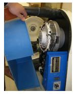
Remove the undercover by removing all undercover screws then sliding the undercover off.
