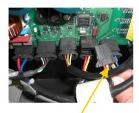
Unclip the other end of the potentiometer from the control board by squeezing the sides of the clip and pulling
