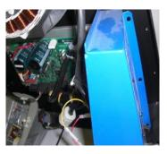
In order to take off the part, the blue panel must be removed in order to unscrew the green ground wire.
