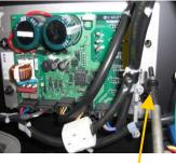
In order to take off the part the control board must be removed to in order to unscrew the green ground wire
