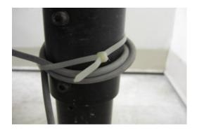
WRAP THE PEDAL CORD SEVERAL TIMES AROUND ONE OF THE FRONT LEGS AND SECURE WITH A ZIP TIE.
