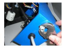
Remove the metal washer from the plastic screw end of the harness
