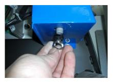
Place the new potentiometer harness in the hole on the blue panel and tighten on with washer
